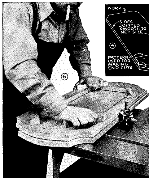
Above, Using a Built-up Outline Pattern for Shaping the Edge of a Small Table Top.
