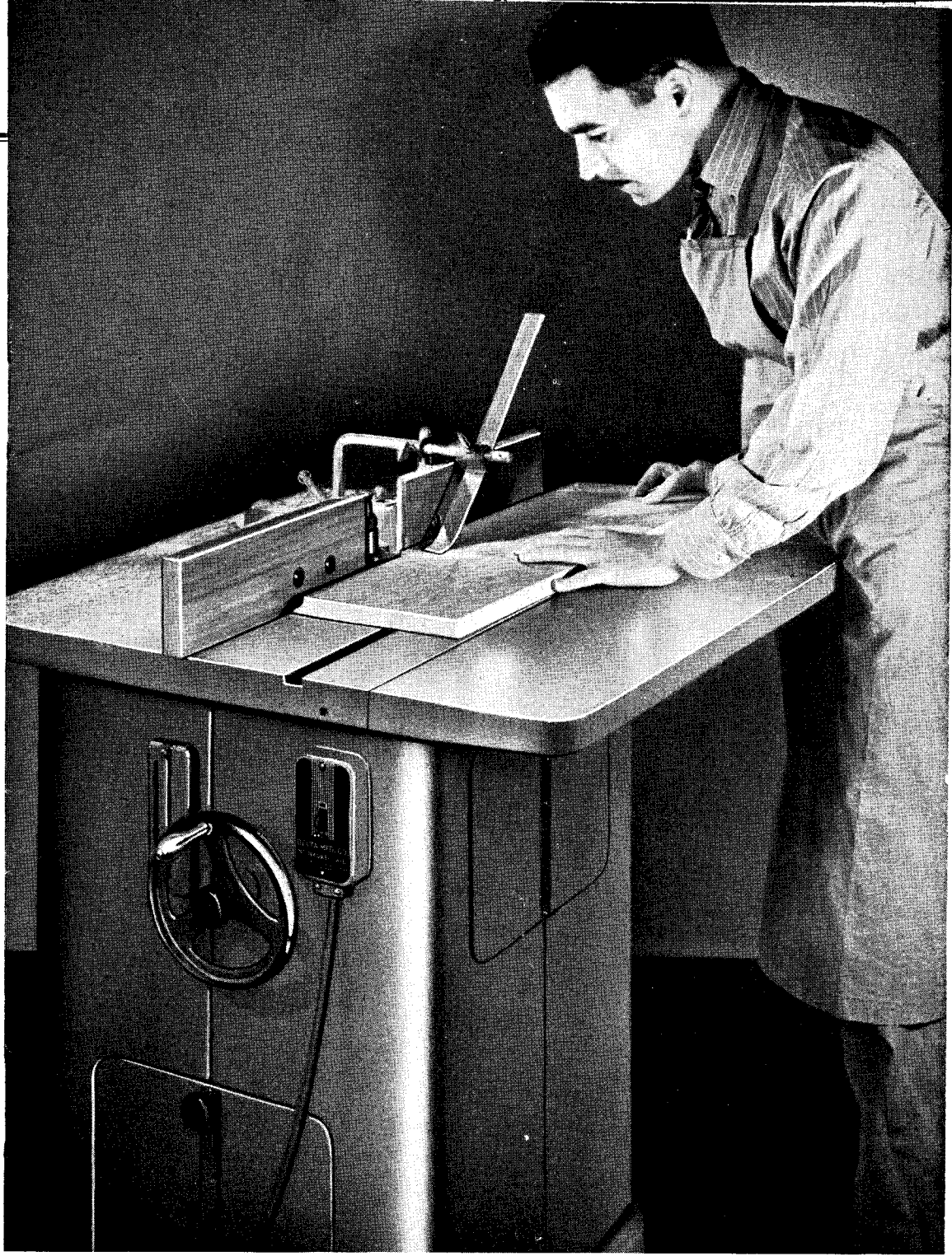
The Shaper... Top Ranking Production Tool for the Small Shop and Capable of a Score of Different Operations, Some of Which are Impossible in Any Other Manner. Photo Above Illustrates Cabinet Model with \frac{3}{4} Inch Spindle. The Machine Should be Located in an Unobstructed Working Space.
